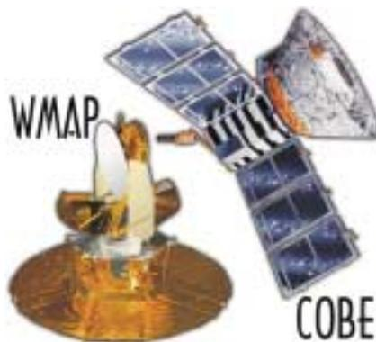
Figure 4 — Representations of NASA’s COBE and WMAP satellite probes, used to detect cosmic microwave background radiation. Images courtesy of NASA.
