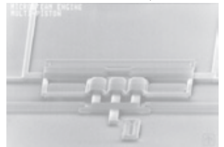
The world's smallest functioning triple-piston steam engine. One piston is five microns across or 1/5080 of an inch.
