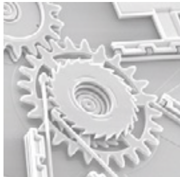
Complex MEMS ratchet mechanism
