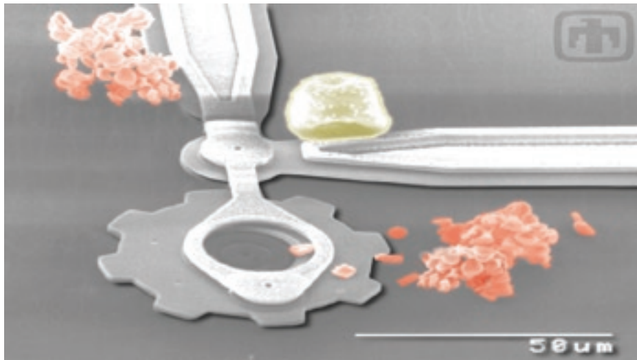
Drive gear chain and linkages, with a grain of pollen (top right) and coagulated red blood cells (top left, lower right) to demonstrate scale.
